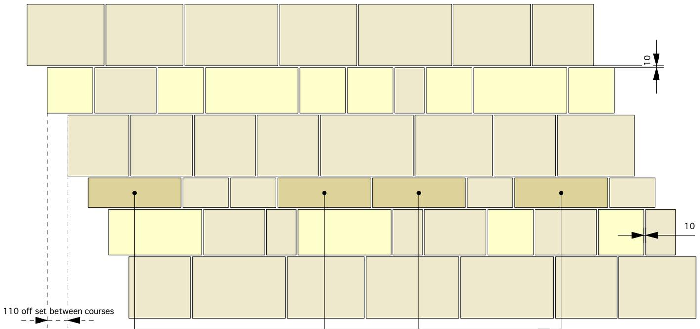
to include a 160 mm course cut 2 pieces of 500 x 330 (from part A stock) in half to create 4 pieces of 500 x 160 or in thirds to create 6 pieces of 330 x 160 pieces or a mixture as required
