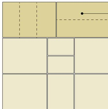
*the Vaucluse pattern is made up of mixed length stone in a variation of course heights of 330, 245 and 160 mm. The pattern can be repeated horizontally and vertically. The bedding joints remain consistent whilst the perpendicular or vertical joints vary.*
