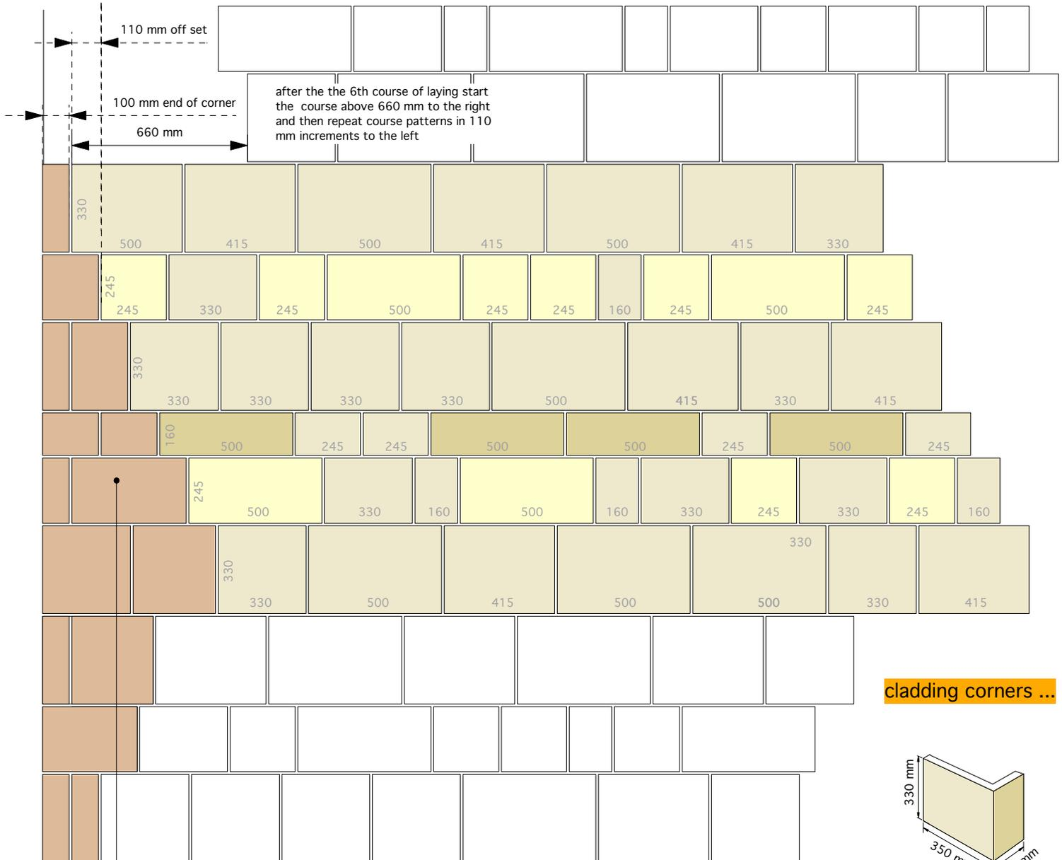
Pieces will need to be trimmed on site as required by the layer to fit external corners, internal edges or end wall finishes. (example of infill only) If using cladding, corner units are available at the same thickness of the stone. Refer diagram attached
